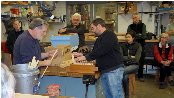
David Eckert demonstrates the value of a frame assembly jig
